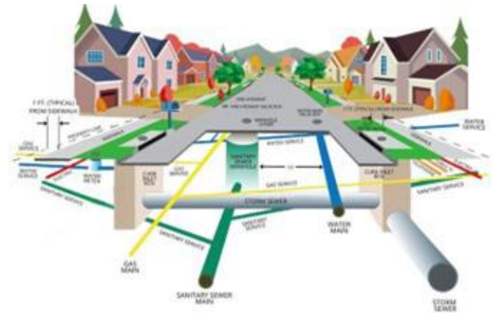
Exhibit 6: A depiction of what typical underground infrastructure looks like within the public ROW. (Prescott Valley/Courtesy)
