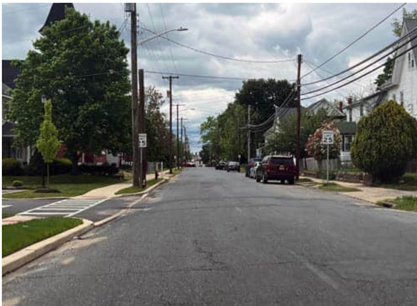
South Avenue has a 29-foot cross section. A faint dashed centerline identifies the two northbound travel lanes.
