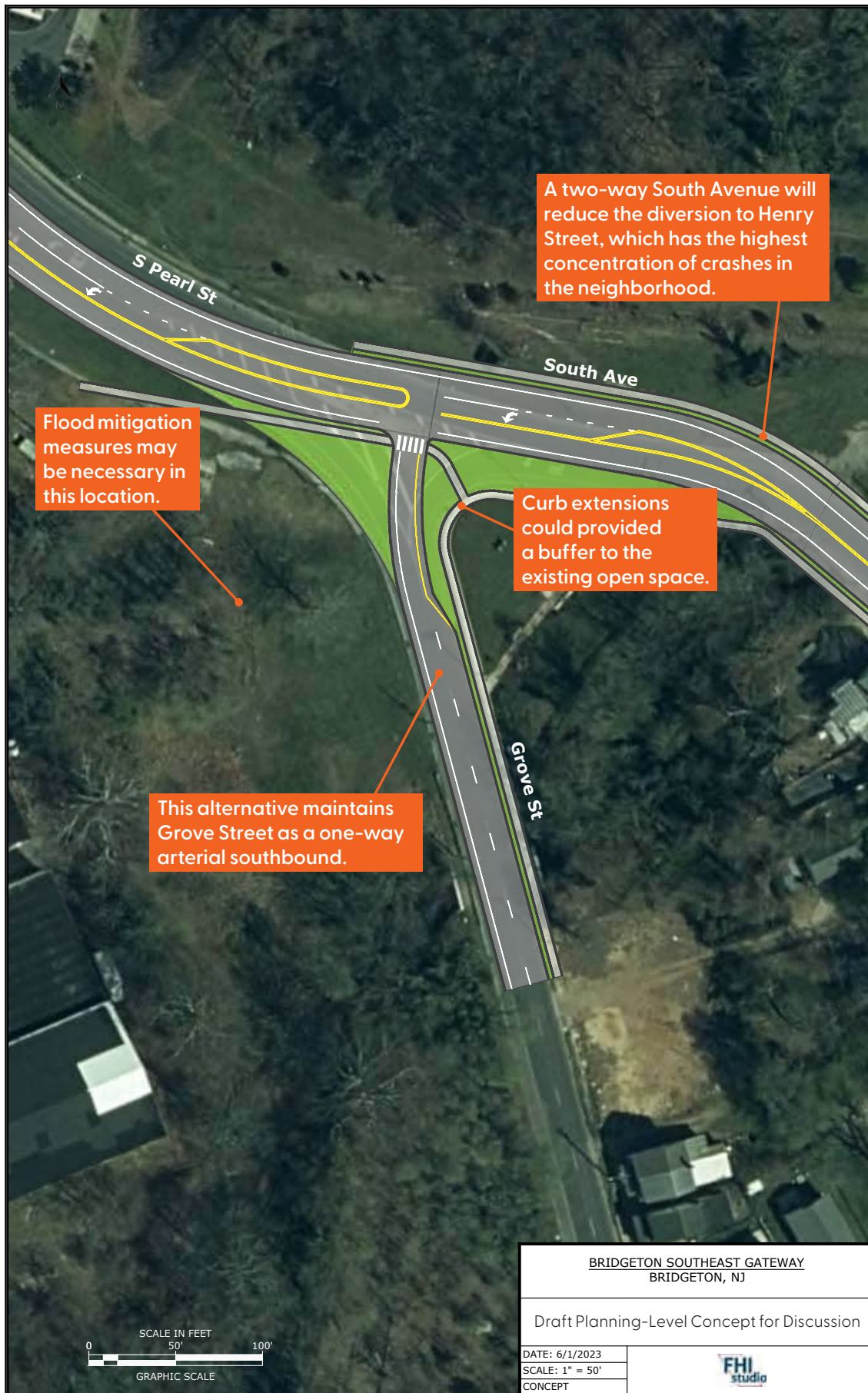
Figure 16. Grove St at South Ave and S Pearl St Minor Realignment Concept Plan
