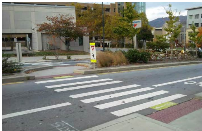
Center crossing islands allow pedestrians to deal with only one direction of traffic at a time. Image: pedbikeimages.org - Lyubov Zuyeva (2011)
