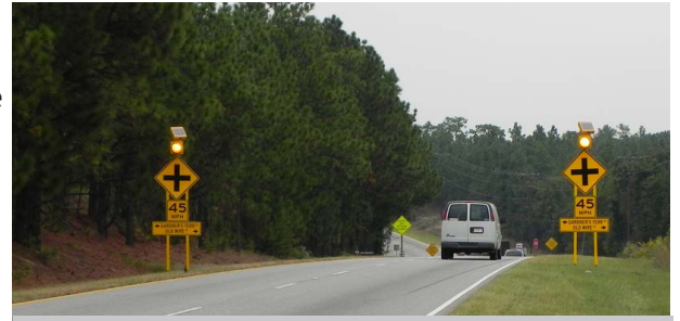
Example of countermeasures on the through approach.
