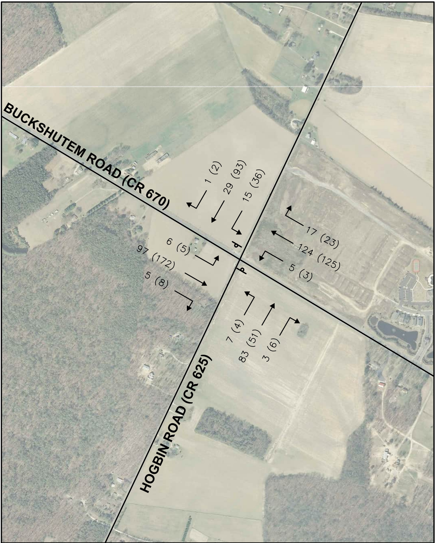
HOGBIN ROAD (CR 625) & BUCKSHUTEM ROAD (CR 670)
